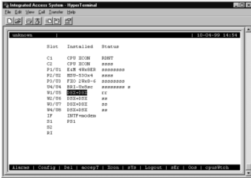
Figure 5-89. Typical Cross-Connect WAN Card Redundancy Switch in Progress
