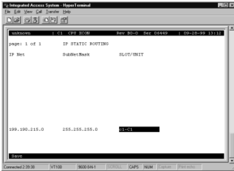
Figure 7-22.IP Static Routing Information Screen
