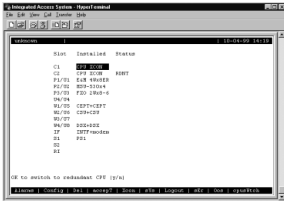
Figure 5-85. Manually Switching to a Redundant CPU
