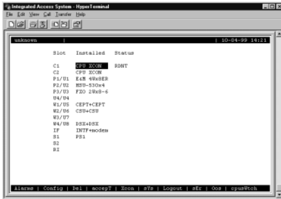
Figure 5-86. Typical System with CPU Switchover Completed
